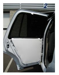
Hinge up window guard and reattach to bracket with 10-32 x <sup>1</sup>/2" Stainless machine screws and #10 Flat washers. **NOTE:** Door panel fillers are provided for the Expedition EL. This is not used for the standard length Expedition.
